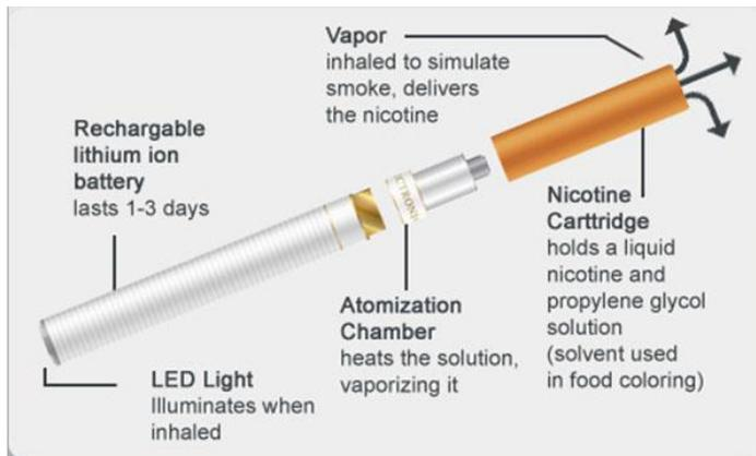
Figure 1. Common Components of ENDS
